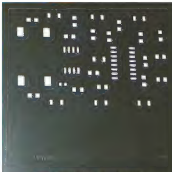
Figure 10. Stainless steel solder mask.
